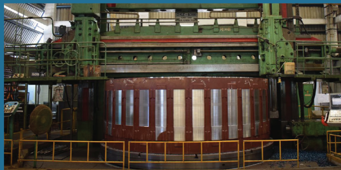
CNC VTL - 6300 mm Dia x 3500 mm Ht
