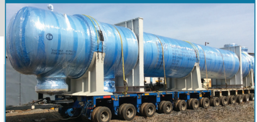
C2 Hydrogenation CC Exchanger Weight: 400 MT (Stacked HX)
