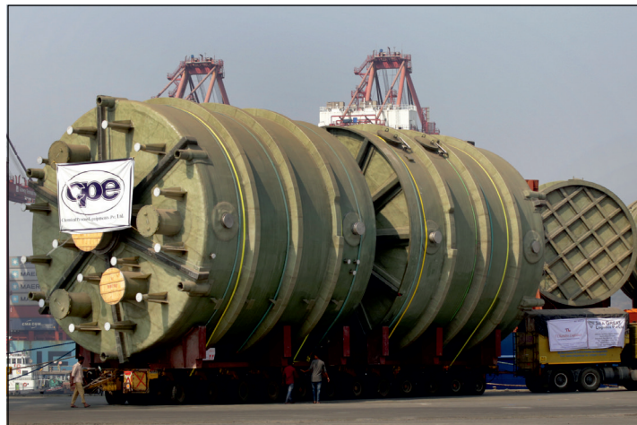
6 Nos. GRP Reactors exported to Singapore (Size: 8.5m Dia x 8.5m Height)
