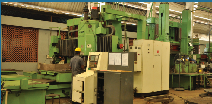
Double Column VMC for Baffle Drilling
